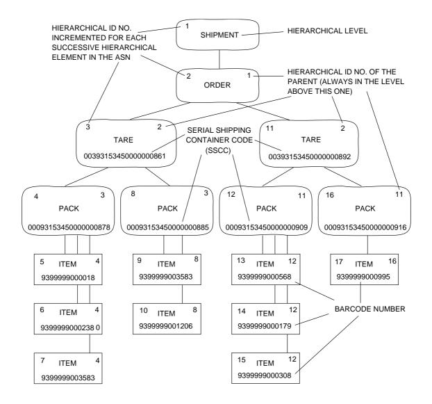
Although the ASN is constructed sequentially in the order shown by the hierarchical ID numbers on the top left corner of each box in the diagram, the conceptual description is better represented by the layout shown.
